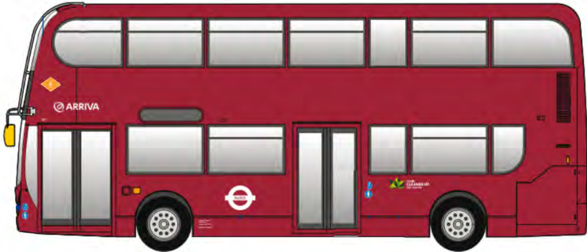
Figure 10_2 Nearside Propulsion Identification Symbol location
